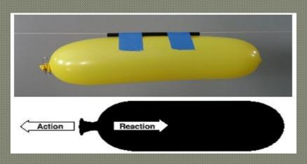
iv) When a rocket is fired, the force of the burning gases coming out (action) exerts an equal and opposite force on the rocket (reaction) and it moves upward
