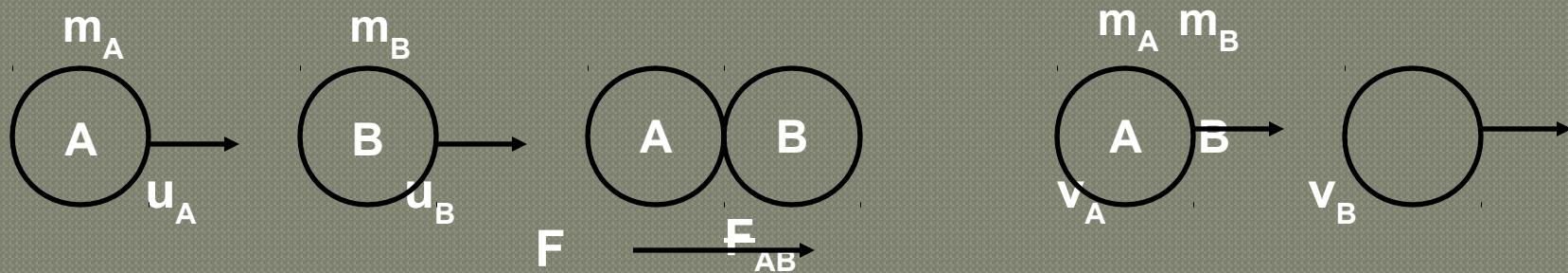
If two balls A and B of masses  $m_A$  and  $m_B$  are travelling in a straight line with initial velocities  $u_A$  and  $u_B$  and if  $u_A > u_B$ , the two balls will collide with each other. During collision at a time t, ball A exerts a force  $F_{AB}$  on ball B and ball B exerts a force  $F_{BA}$  on ball A. If  $v_A$  and  $v_B$  are the velocities of balls A and B after collision,
