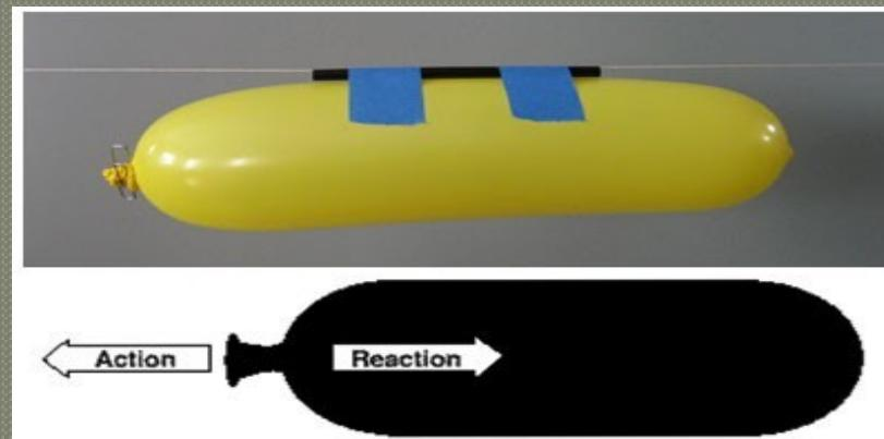
iv) When a rocket is fired, the force of the burning gases coming out (action) exerts an equal and opposite force on the rocket (reaction) and it moves upward.
