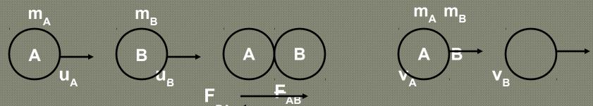
If two balls A and B of masses  $m_A$  and  $m_B$  are travelling in a straight line with initial velocities  $u_A$  and  $u_B$  and if  $u_A > u_B$ , the two balls will collide with each other. During collision at a time t, ball A exerts a force  $F_{AB}$  on ball B and ball B exerts a force  $F_{BA}$  on ball A. If  $v_A$  and  $v_B$  are the velocities of balls A and B after collision,
